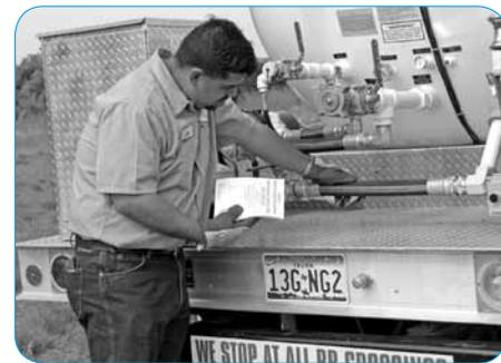
*Inspecting Hose Reels, Meter and Connecting Piping*
