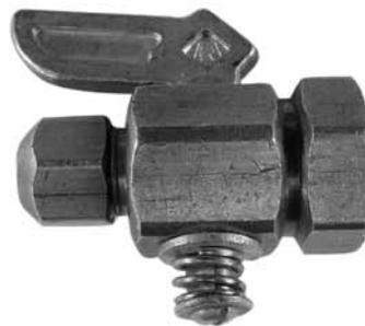
**Figure 2** Unapproved shutoff valve. The spring and nut are located outside the valve body.
