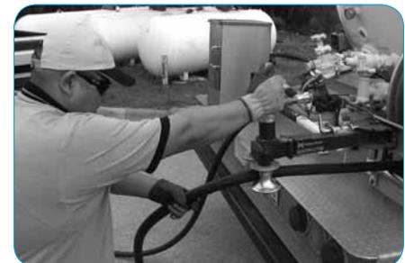
*Inspecting Delivery Hose Assembly After Each Delivery*
