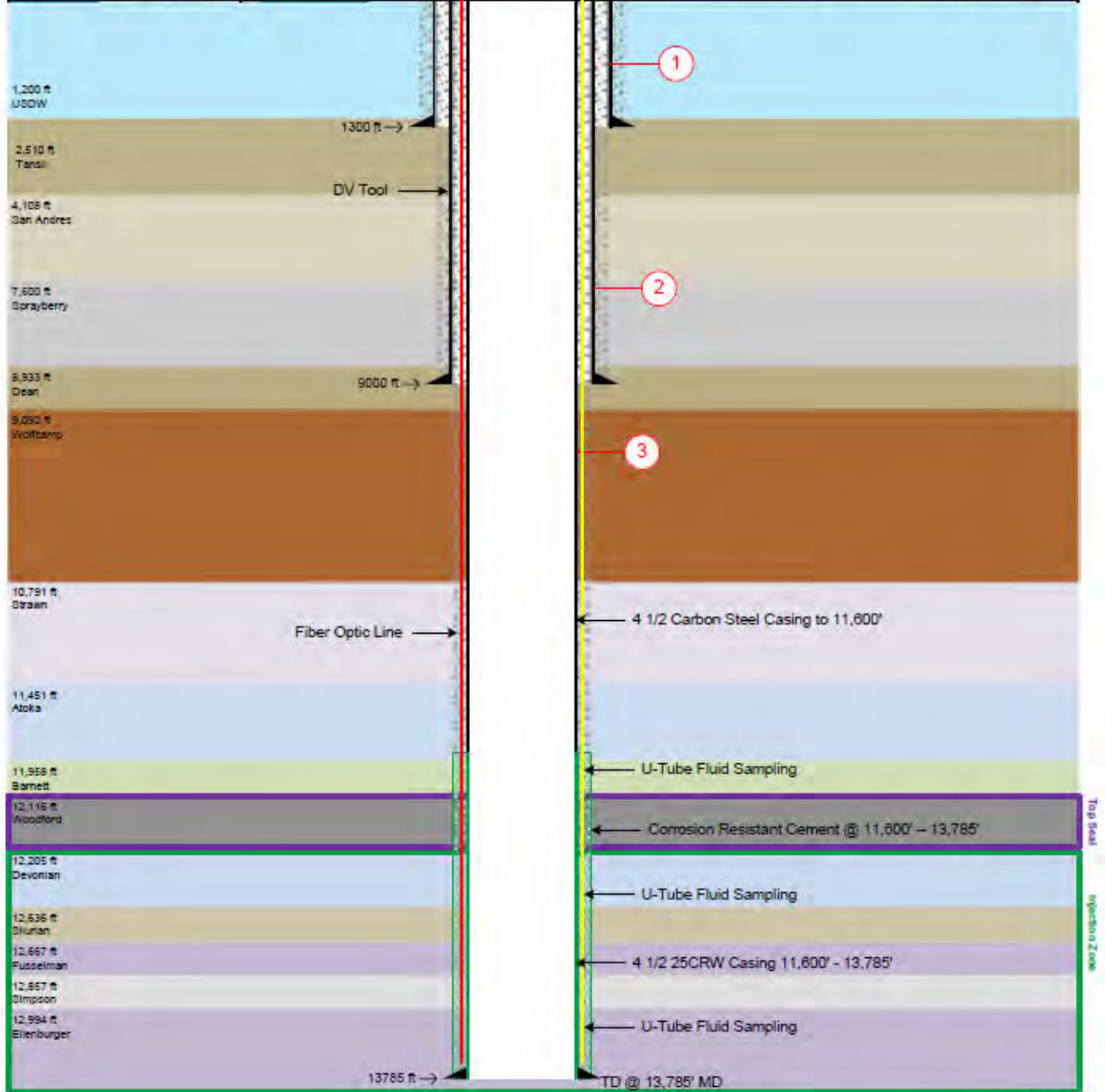
Figure 3-11: Midland IZM #2 Wellbore Schematic
