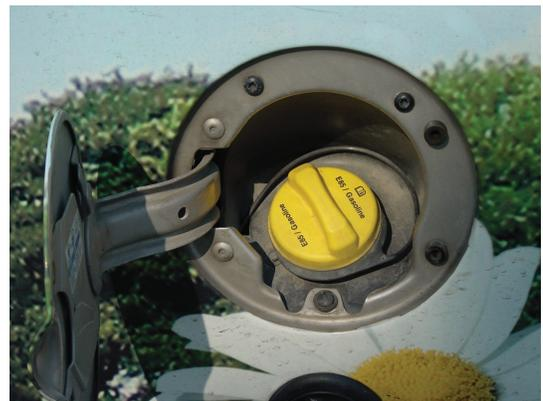
Figure 32. Bi-Fuel Vehicle Gasoline Fill Connection
