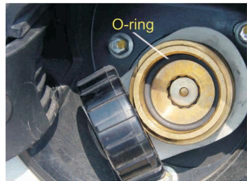
Figure 38. Filler Valve O-Ring
